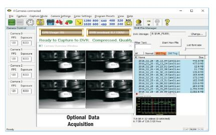
The Mega Speed MS 35K PRO camera control software is a complete software package that is included with each system. With the camera control software you can simultaneously adjust the camera settings, record the process, review the recently recorded events, edit, play back, review and transfer files without interrupting the recording process.
