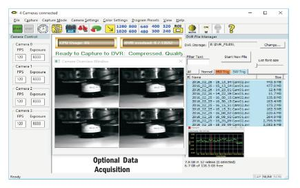
The Mega Speed MS 35K Fiber camera control software is a complete software package that is included with each system. With the camera control software you can simultaneously adjust the camera settings, record the process, review the recently recorded events, edit, play back, review and transfer files without interrupting the recording process.
